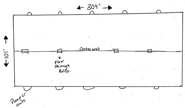
This Pit is 101' x304' and is 8' deep. the concrete is reinforced with rebat. There is a center support wall in the middle and there is 4 flow throughs at the bottom of the center wall. There are also 5 pump outs (PTO driven Certrificals) on each side of the building. The floor is 100% total slats.
